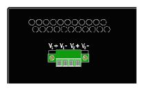
Unscrew & Remove the DC Voltage Input Plug from the Power Input Header Install the DC Power Cables into the Plug (observing polarity). Plug the Voltage Input Plug back into the Power Input Header. Tightening torque for the terminal block power plug is **0.22 Nm/0.162 Pound Foot**. Verify the Power LED stays ON (GREEN).
